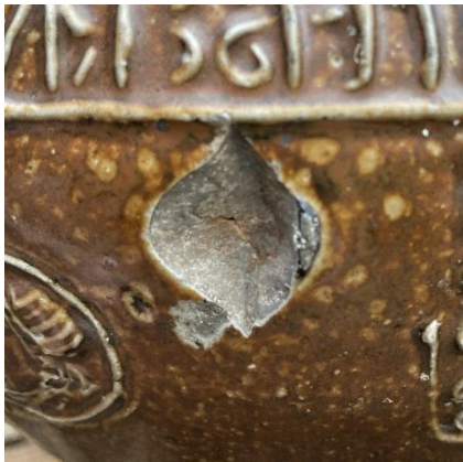
Cavity in surface of pot, believed to have been caused when breaking a glaze bridge with an adjacent pot, formed during firing
