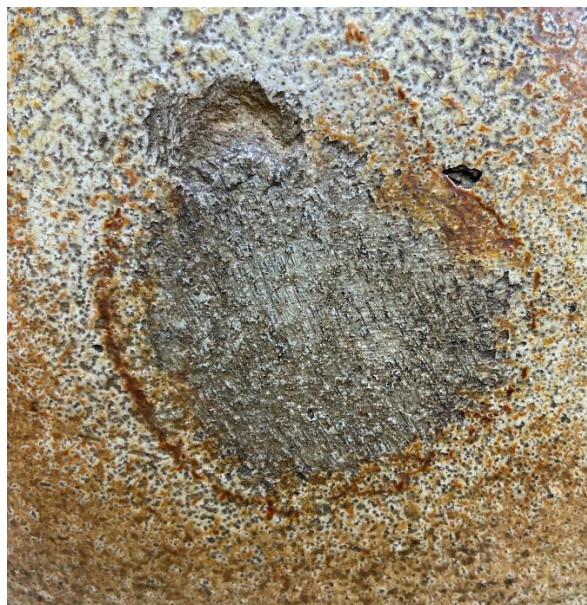
Stacking scar and separation damage (scar is 3 cm across)
