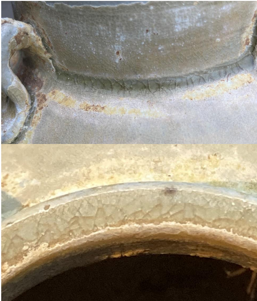
Areas of thicker glaze near rim, showing crazing
