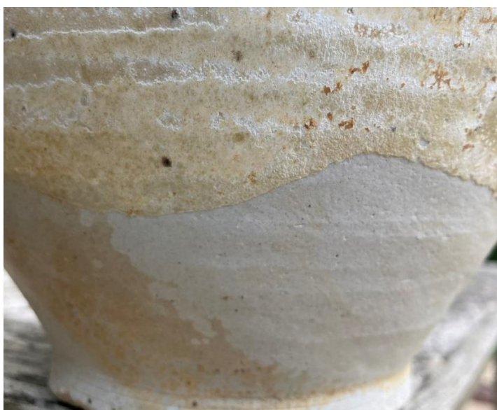
Bare clay body bottom right, white slip coating top, remnants of glaze on left and on slip
